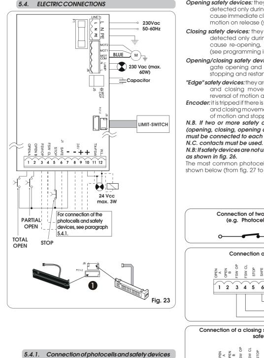
Before connecting the safety devices and photocells we advise you to select the type of operation according to the movement area they have to protect (see fig.24 for example):
